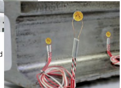
Railway axle load measurement
