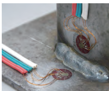
Weld bead (rosette strain gauge)
